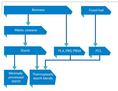
Figure 5.2 Simplified schematic of the production of starch-based polymers
