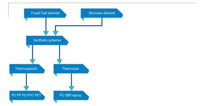
**Figure 2.2** Production of conventional synthetic plastics from fossil fuel and biomass sources (adapted from Joint Group of Experts on Scientific Aspects of Marine Environmental Protection 2015)
