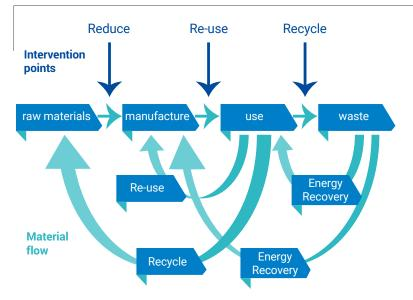
**Figure 2.8** Closing the loop within the plastic economy, showing options for re-using, recycling and recovering energy, within the globally-understood 3 Rs principle of Reduce, Re-use and Recover (adapted from United Nations Environment Programme 2016).
