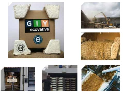
Figure 4.5 Production of Mycofoam<sup>™</sup> from agricultural waste, showing the raw material, inoculation by a fungal strain, incubation and pressing. The example shows protective corner mounts, replacing the use of EPS; images courtesy of Ecovative.
