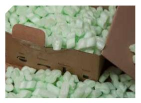
Figure 2.14 Loose fill used to protect goods in transit, made from EPS, ©Peter Kershaw.
