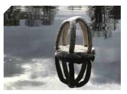
Figure 4.6 Grown structures created using waste cardboard, cotton bandage and inoculation with oyster mushroom mycelium – practical and edible; images courtesy of the Mandin Collective.
