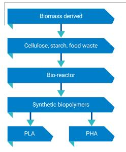
Figure 5.4 Simplified schematic of the production of poly(lactic acid) (PLA) and polyhydroxylkanoates (PHA).
