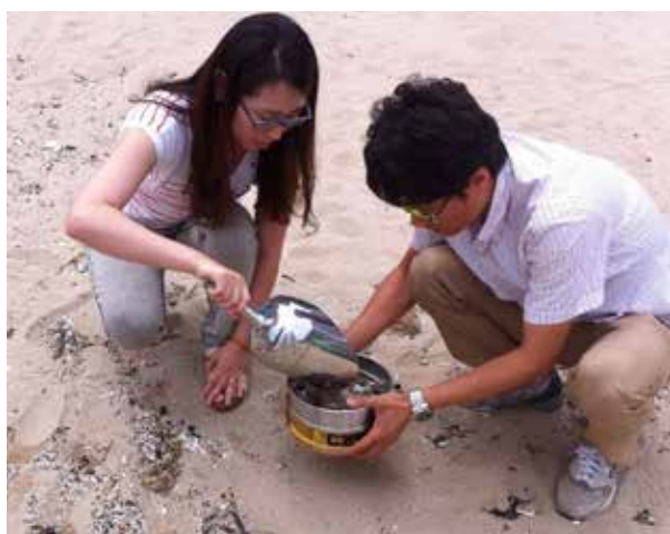
Figure 4.14 Sampling surficial beach sediment to collect resin pellets for chemical analysis, using a coarse and a fine mesh sieve, 2014 near Busan, Rep. Korea (© Peter Kershaw).
