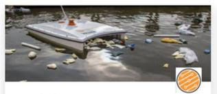
WasteShark™ Autonomous drone called Waste Shark removes plastic waste and contaminants from water bodies
