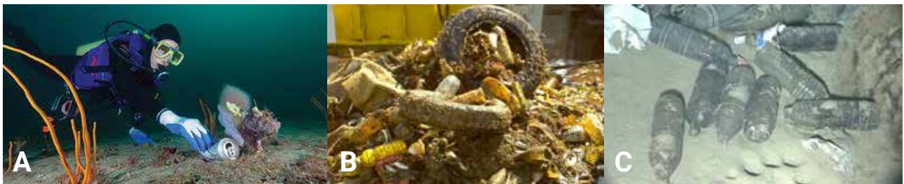
Figure 4. Common approaches to monitor mega and macro litter at the bottom. Diving in shallow waters of US west coast (A; >30m), trawling on soft bottoms of the NW Mediterranean sea (B; 50m) and Remote Operated Vehicle on rocky/mixed bottoms (C; 1000m) (Source: NOAA; IFREMER).
